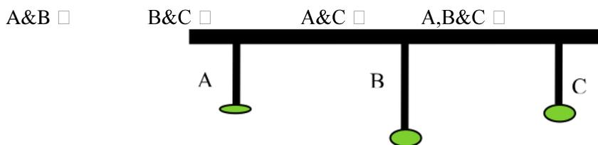
(21) Nora and Omar set up the circuit shown alongside. They predicted that, when they closed the switch, bulb B would light up and bulb A would be unaffected.
